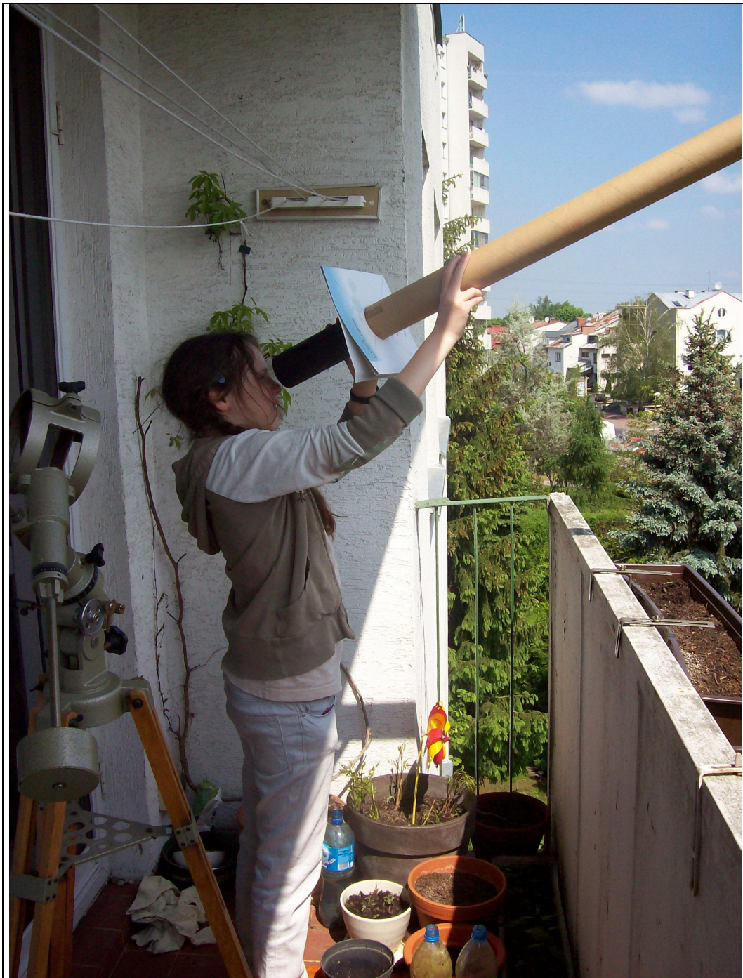
Pic. 10. Observations, aim the pinhole at the Sun and watch it on the focusing screen
