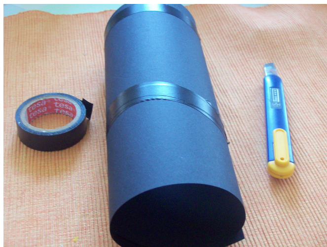
Pic. 8. A black cardboard tube ready to be put onto the focusing screen for additional cover from the sunlight.
